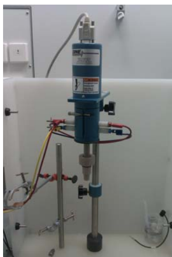
Figure 2 Apparatus for rotating disk electrode measurements.
